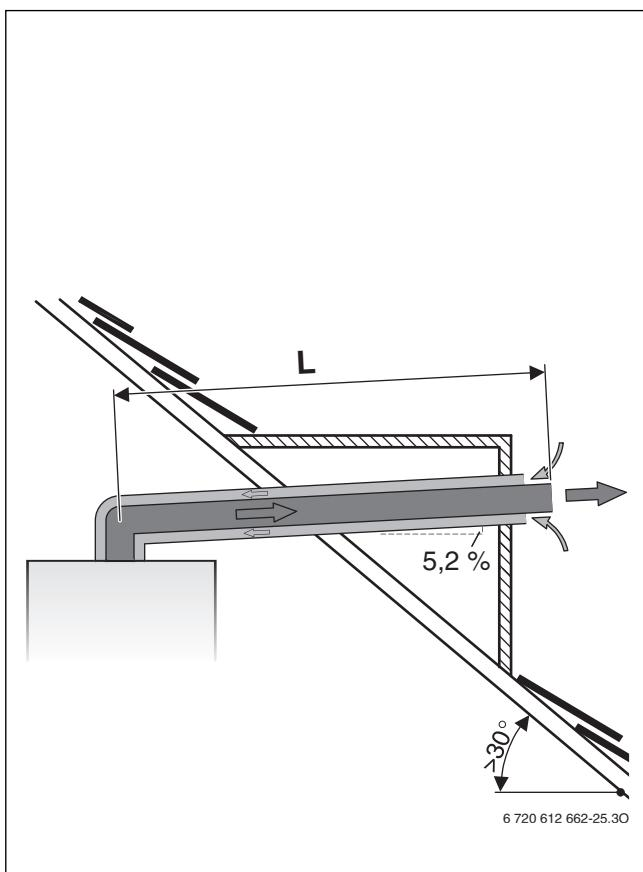
Fig. 12 Ghidarea gazelor arse pe orizontală conform C<sub>13</sub>
